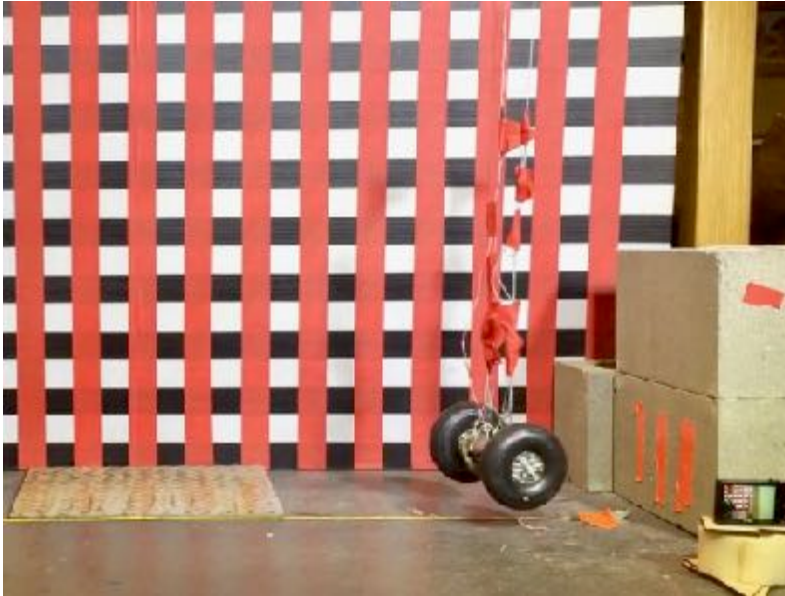
A weighted rig was used to simulate forces from high altitude drops, with an accelerometer and slow motion camera measuring impact severity.
