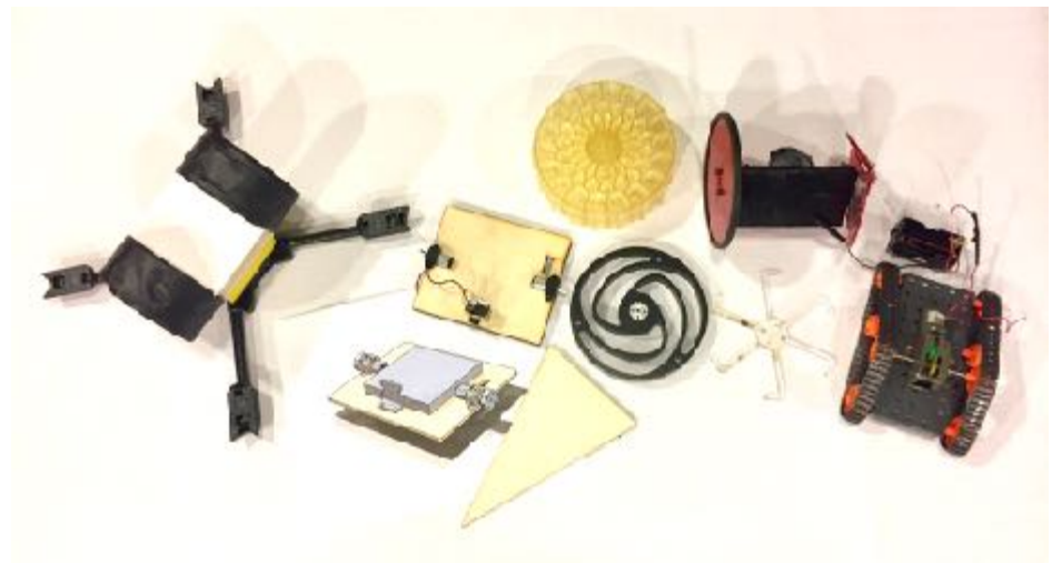
Early prototypes for sizing, mobility, and drop tests
