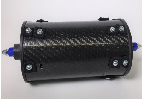
Figure 8: Chassis assembled with fasteners in place
