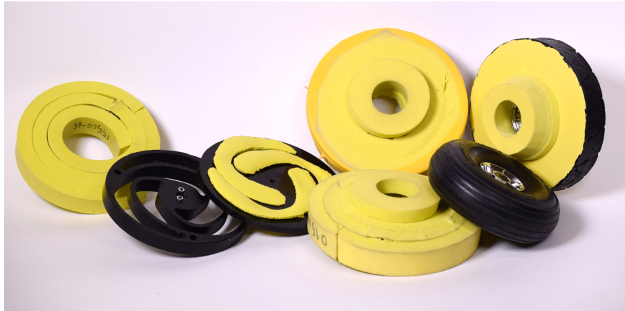
Figure C.3.1: Wheels from left to right: PORON® XRD® 15500-65 Strips; the original Nylon Suspension Wheel; Nylon Suspension Wheel with PORON XRD 12500-65 inserts; (above) 09500-65 Disks with Side Impact Protection; (below) 09500-65 Strips with Side Impact Protection; Pneumatic Wheels; Final PORON® XRD® 09500-65 Disk Wheels.
