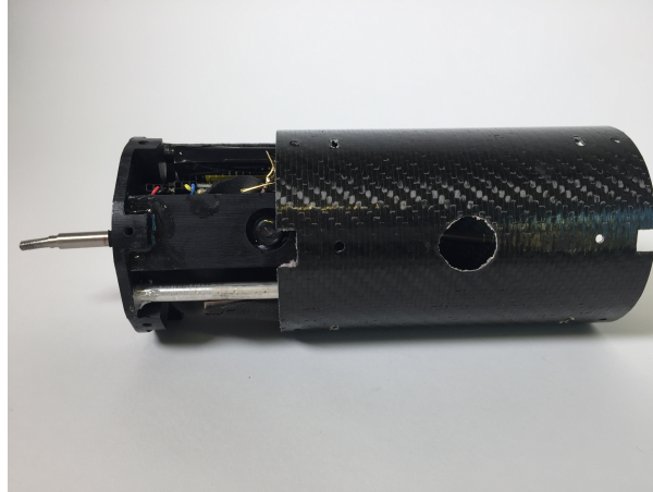
Figure 6: Sliding the inner chassis into the carbon tube
