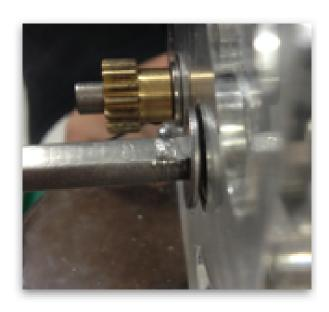
driveshafts were not actually hardened, causing them to deform under the pressure of the set screws (see above).
