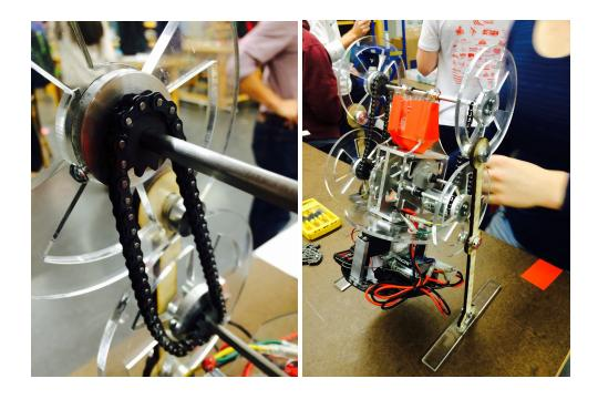
The turning mechanism also had limitations. The wires connecting the motor to the power could catch while the bottom plate was spinning, either because they were at the end of their rope, or because they got tangled. This would stall out the turning, and required the driver to take time to unwind the wires, effectively resetting the turning mechanism.
