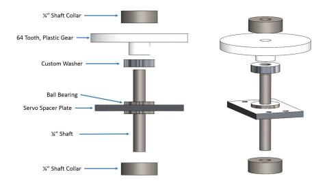
First the shaft was inserted into the ball bearing pressed into the servo spacer plate. The 64 tooth, plastic gear was aligned with the gears on the servos using a fabricated washer. Then a ball bearing in the center of the top plate was put over the shaft. The shaft was held in place by
